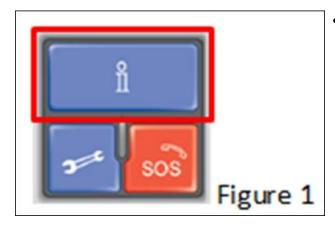
First attempt to verify the customer complaint by pressing the "i" button (see Figure 1) in the overhead console.
