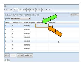
Under Hex Input <arrow 1>, select the blank box <arrow 2> that lines up with the byte to be changed (e.g. "0" shown).
