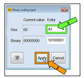
**Tip:** The binary coding input pop-up window allows for coding corrections.
