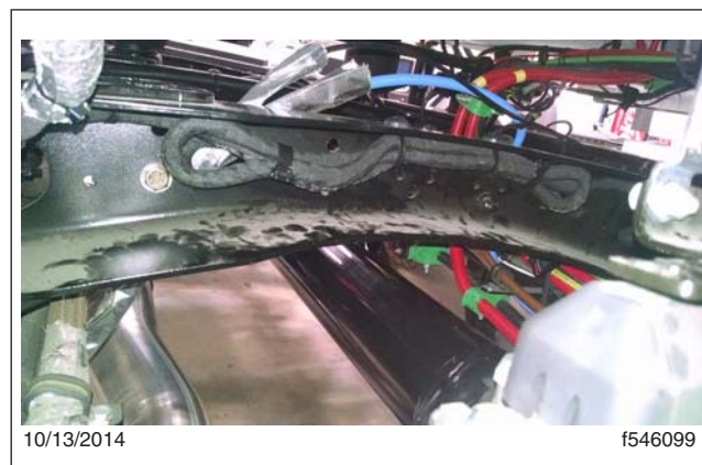
Fig. 6, Harness Secured in the Crossmember with nylon Cable Ties, Part Number 23-12069-001
