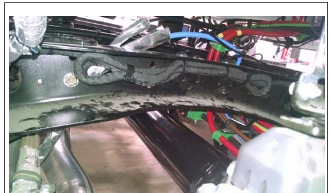
Fig. 6, Harness Secured in the Crossmember with nylon Cable Ties, Part Number 23-12069-001
