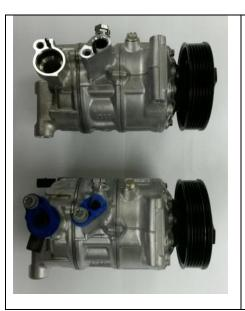
When installing the new AC compressor immediately transfer the AC compressor caps to the original compressor as shown.
