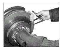
Technician must record the final thickness measurements on the back of the repair order.
