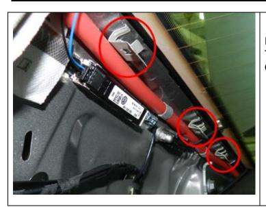
Install them in the proper location along the glass. This makes the installation and alignment of the C-pillar much easier.
