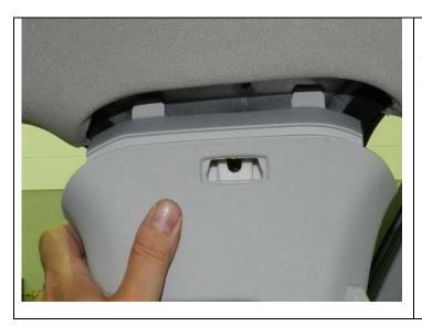
The B-Pillar installation is difficult and can affect the headliner fit and finish.
