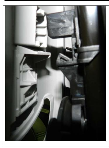
After the screw is installed, Align the B pillar trim seatbelt adjustment lever with the seatbelt adjustment mechanism on the B- pillar.
