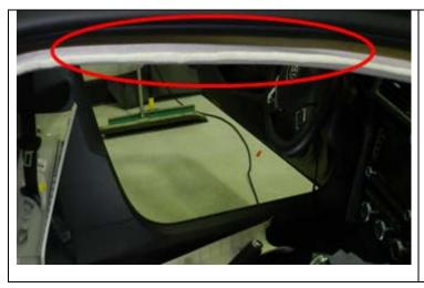
Once all the trim is installed make sure that the headliner and trim edges are properly tucked behind the door seals.
