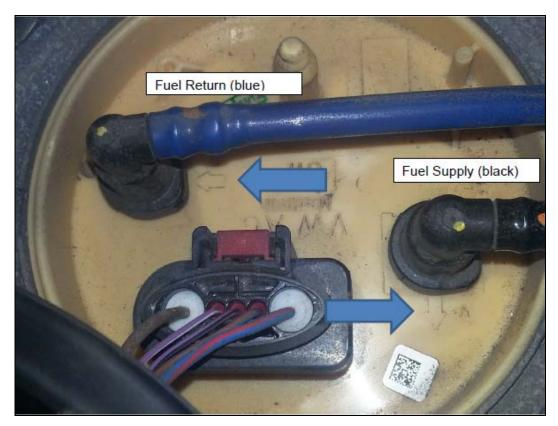
On 2009-2013 Common Rail Diesel Engines with a whining noise from the auxiliary fuel pump, verify correct fuel line installation at the in tank fuel pump. Additionally, verify correct line installation at the fuel filter (compare to a like unit or Elsa Repair Manual).
