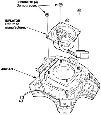
8. Use shop air to clean any debris that may be on the inflator, then remove the inflator from the airbag.
