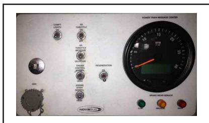
Figure 18 - Engine Control Panel
