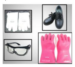
**5. NEVER** use insulating gloves that have expired. Prior to each use of the insulating gloves, confirm that the certification date, stamped on the gloves, is within 6 months of the current usage date. The gloves need to be recertified after every six months of use by an approved facility. Check the gloves for cracks, tears, or damage by rolling the gloves to check for air leaks. Do not use any leaking gloves.
