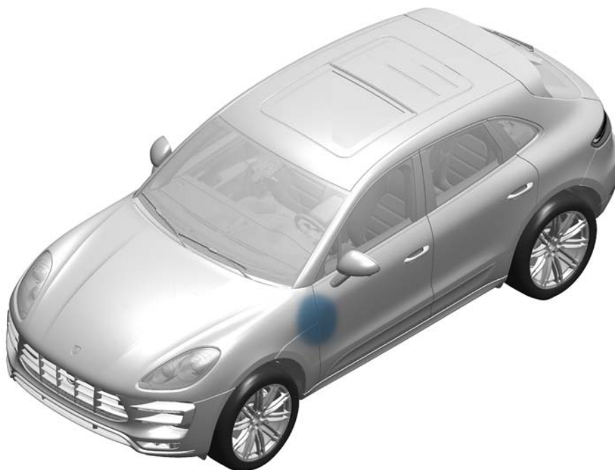
Checking gap dimension of front door
