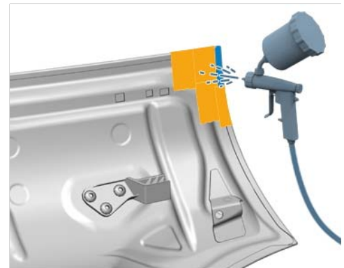
Reworking flange seam on lid
