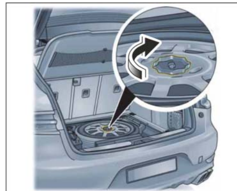
Storing collapsible spare wheel in luggage compartment pan
