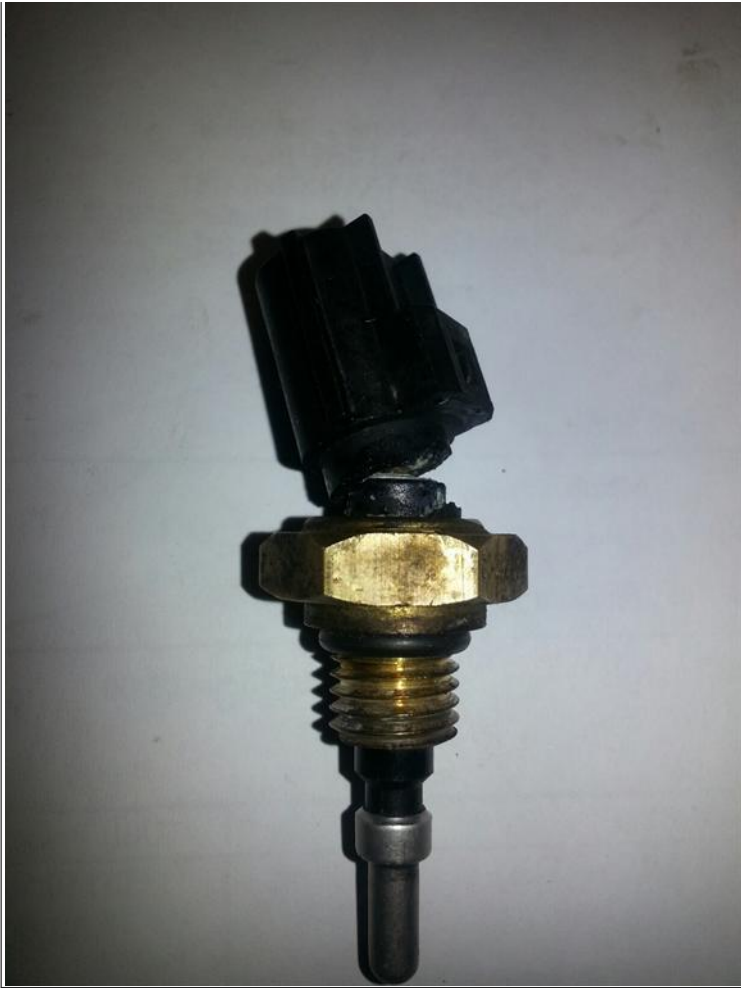
Figure #1: Broken CACOT Sensor
