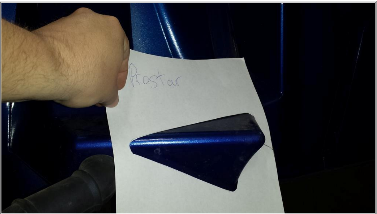
Figure #2: Hood Rubbing Mark From Sensor
