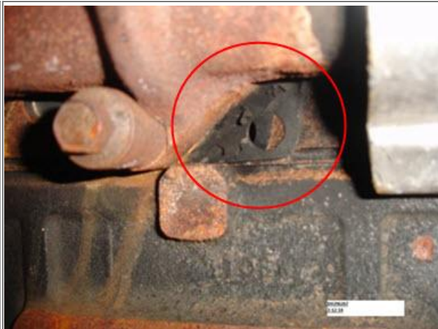
Figure 2 - "Bad" manifold gasket, bottom of cyl. #3
