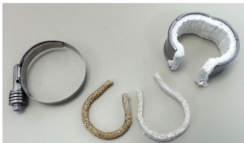
Figure 7 - Cuff Seal Assembly (broken down)
