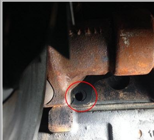
Figure 1 – "Good" manifold gasket, bottom of cyl. #3
