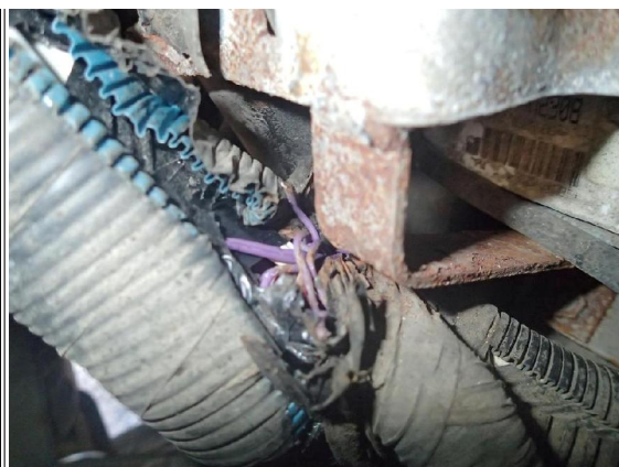
Figure #2: Harness chafing(incorrectly routed)
