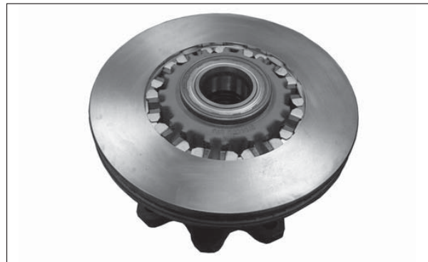
FIGURE 90 - INTERMEDIATE ELEMENTS (SPACERS) INSTALLED
