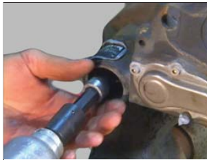
FIGURE 67 - REMOVE THE CALIPER BOLTS
