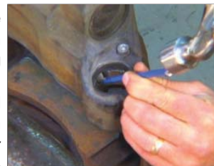
FIGURE 73 - REMOVE THE TAB THAT HOLDS THE BUSHING IN POSITION
