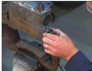
FIGURE 78 - POSITION THE NEW BUSHING
