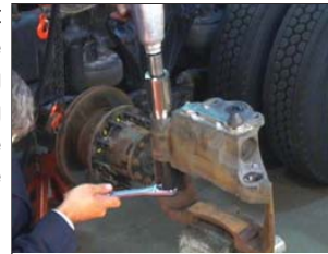
FIGURE 71 - REMOVE THE LONG GUIDE PIN
