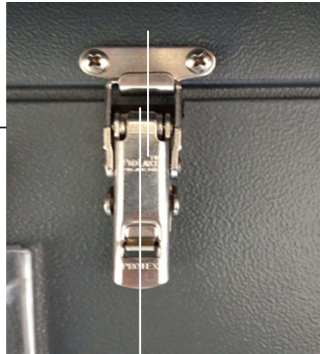
Figure 1 - Latch Location and Misalignment
