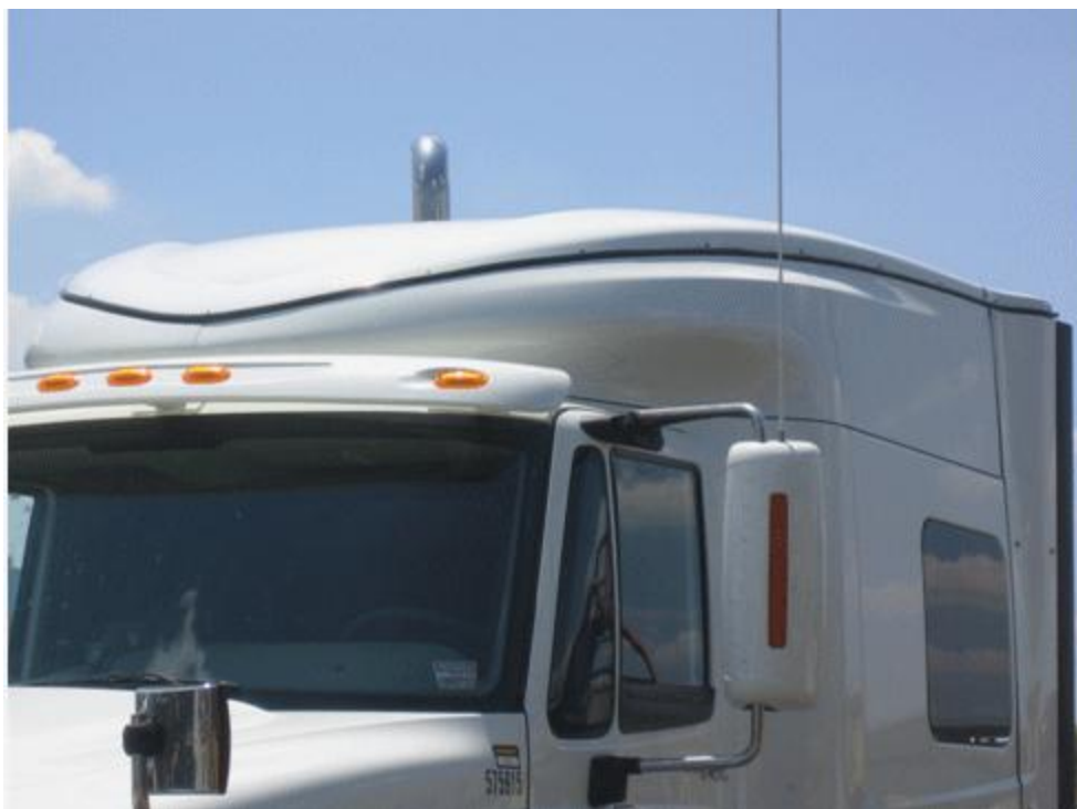
Photo 2. Installation of the seal is complete. Only the creation of water drains remains.
