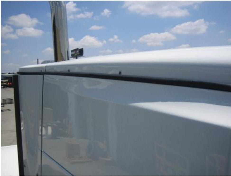
Photo 1. The black, D-shaped seal is adhered to the roof under the air deflector mounting nuts and above the roof lip.
