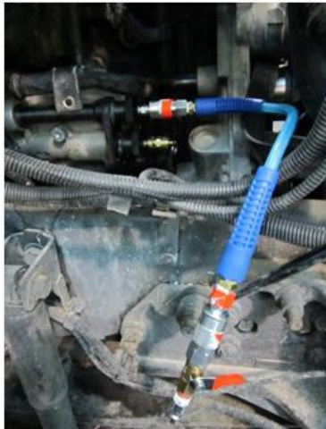
Figure 5: Air hose extension and fittings installed in chassis
