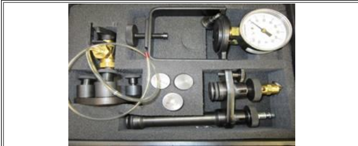
Figure 2: KL20030NAV - EGR Cooler Leak Detection Kit
