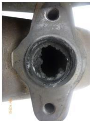
Figure 2 – Partially plugged AFI port
