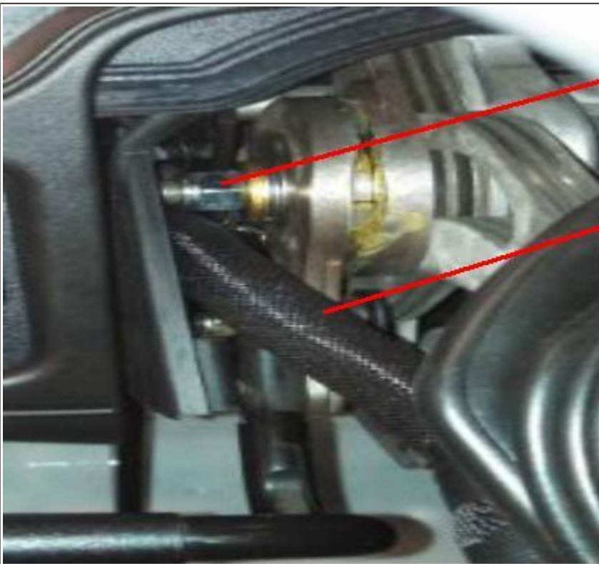
Figure 2: Correct Harness Routing Inspection Point 1.
