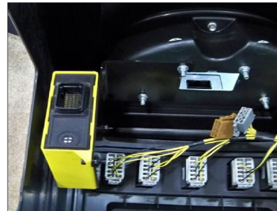
The DAM is the yellow module located behind the console under the I-Pack. The view is with the console removed.
