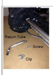
8. Install Head Unit back into the DEF tank, taking care to not force it in. Look through the filler neck and verify that the bottom of the DEF head assembly is located on the alignment feature (appears like a black ball). Reinstall screws.
