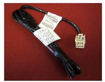
Connect the harness to the MID-BEC (X61A). The MID-BEC is located under the I/P to the left of the steering column. The harness connection point (1) is illustrated below
