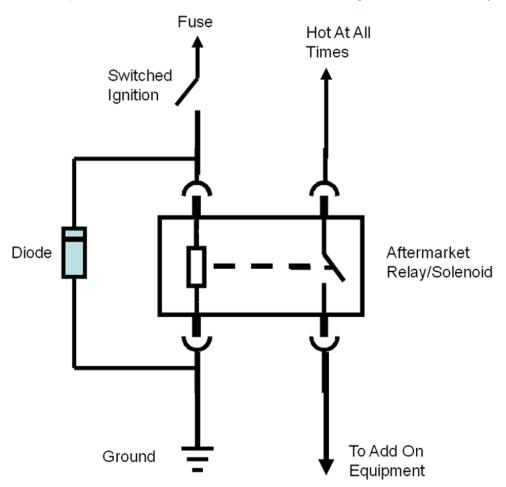
Install a diode, P/N 12112422, across the coil of the relay. It is important that the striped end of the diode be connected to the positive terminal of the coil and the other end of the diode be connected to ground. Be sure to insulate the diode with heat shrink tubing before installing.
