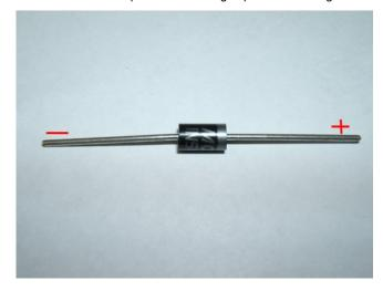
Install a diode, P/N 12112422, across the coil of the solenoid. It is important that the striped end of the diode be connected to the positive terminal of the coil and the other end of the diode be connected to ground.
