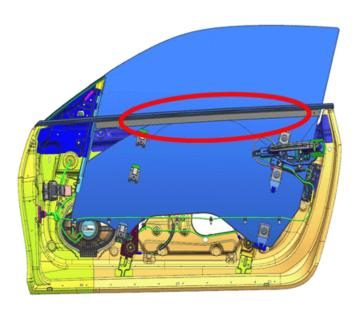
Check the forward run channel seals to make sure they are not folded under the forward edge of glass. You cannot see this unless you look down through the belt line seals
