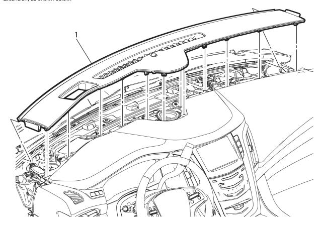
The HUD shroud may have four areas with felt tape (1), as shown below, which is inadequate to eliminate this noise.
