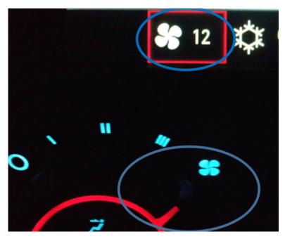
To confirm this, rotate the blower motor knob back and forth while watching the data display menu of the HVAC module in GDS2. The requested fan speed will change up and down correctly in the scan tool as the knob is rotated on the center stack.
