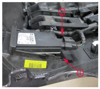
• Identify if the left or right side object sensor module (1) is not retained in the bracket properly and identify if the module's connector (2) is not fully seated.
