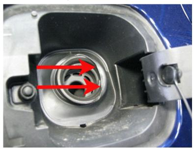
If the rubber is rolled over the filler neck, roll the rubber back over to the correct position. Check fuel filler cap to make sure the seal on the cap has not been damaged.
