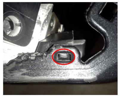
While the fascia is removed, remove the flashing if any, and install the fascia to see if removal of the flashing resolves the issue. If flashing is not the cause or has been removed and the fascia clip still does not fully engage into the bracket, the bracket may need to be replaced.
