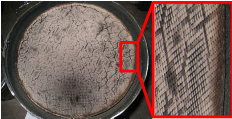
Cut Away View Of Distressed DOC
