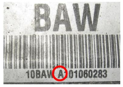
If there is an "A" before the sequence number then replace the OCV/Cam Actuator Solenoid Valve with a replacement "service" valve.
