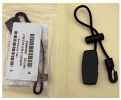
To install the guide, connect it to the loop sewn in the rear outboard seat locations, as shown below.
