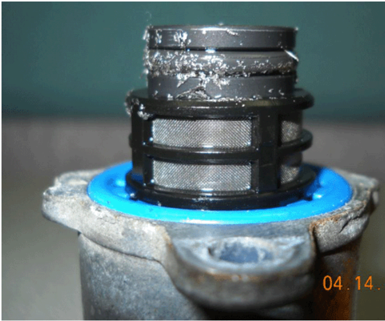
Contaminated Fuel Pressure Regulator 1 (View C)
