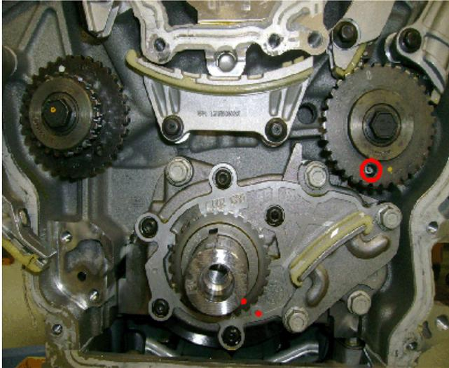
Stage one primary chain alignment for the crankshaft and the left intermediate gear are shown below. The intermediate gear has a triangular shaped timing mark that aligns with the painted link and the crankshaft has a dot to dot alignment.
