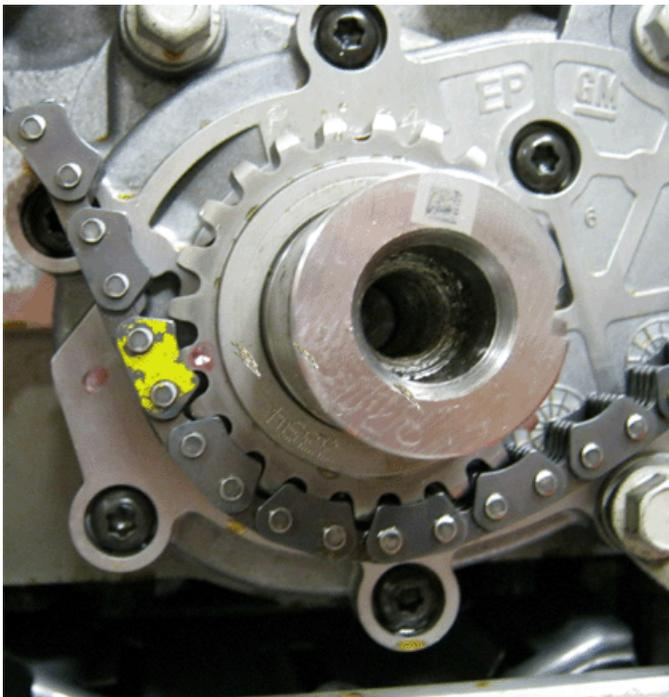
EN 48383-3 should be installed on the right bank or bank one. The triangular marks should be aligned as shown.
