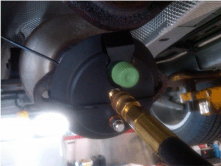
If a leak is found in these areas along with gasket replacement, filing the mating surface of the pipe is suggested.
