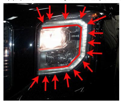
To inspect the halo ring light operation, perform a cold engine start and turn on the headlight switch to the "park" or "headlight" position. Make sure the left and right front park halo ring lights stay on steady. If any of the halo ring lights flicker or operate erratically, perform normal diagnostics. If root cause cannot be determined, replace the affected headlight.
