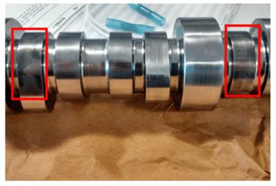
If the date code is 13360 or 14-01-14 these would be suspect camshaft.
