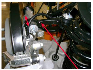
Use a pry bar and apply forward and rearward pressure to the bushings at the spindle end. Also test at the frame end.
