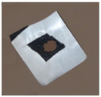
6. Add two <sup>3</sup>/<sub>4</sub>" by 1 1/2 " long by 7/16" thick of Kent Adhesive Backed Shim Stock (foam) p/n P46505 or equivalent centered between the retaining clips on the leading edge of the package shelf (behind/under the rear seat back) see picture below.
