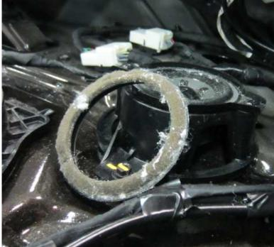
2. OnStar module - place 1/4" foam pad underneath the module (if foam is not currently in place). Use (4) 1" x 6"x 5/16" thick strips of Kent Adhesive Backed Shim Stock (foam) p/n P46510 or equivalent. Note: Do not apply foam the beyond the base of the module, avoid adding the foam in the area of the mounting flanges.
