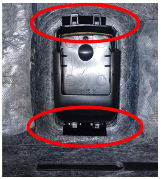
Add foam grommets onto each of the Christmas tree fasteners (if not present) prior to reinstalling back into the package shelf sheet metal holes. Use 1" X 1" block of Kent Adhesive Backed Shim Stock p/n P46510 or equivalent to create a foam washer(s) as needed. Fold the 1" x1" block over from corner to corner and carefully cut a hole in the center of the block to create a washer/spacer, see pictures below.
