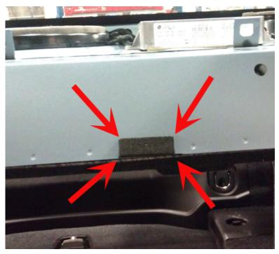
7. Check the "J" hooks of the package shelf cover/trim for being secure. See picture below. Use hot glue to resecure the "J" hooks as needed.
