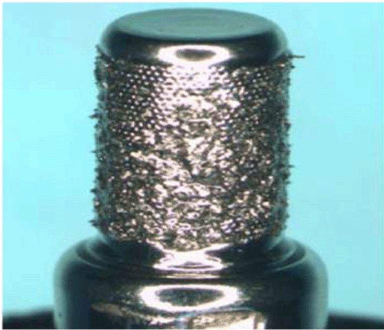
Contaminated Fuel Pressure Sensor
