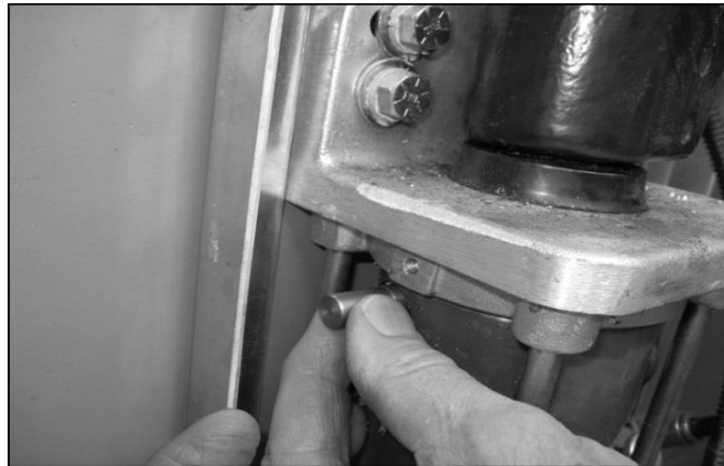
Figure 8 - Round Gage Installation to Rotary Operator
