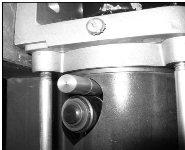
Figure 8 - Round Gage Installation to Rotary Operator
