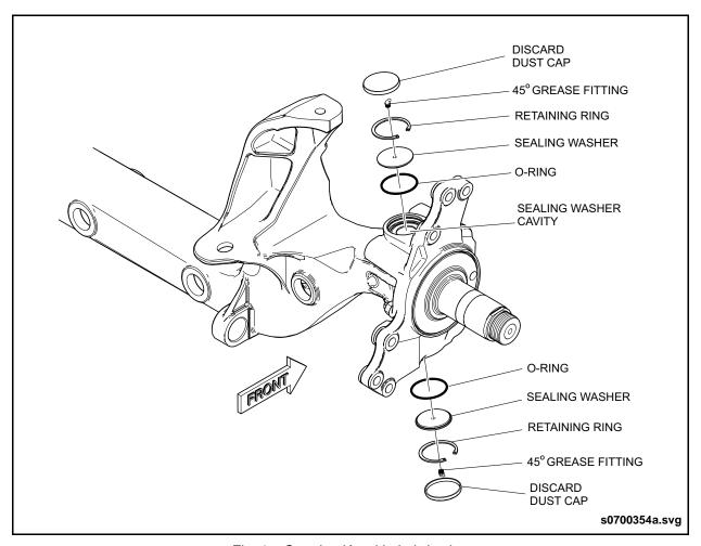
Fig. 1: Steering Knuckle Lubrication
