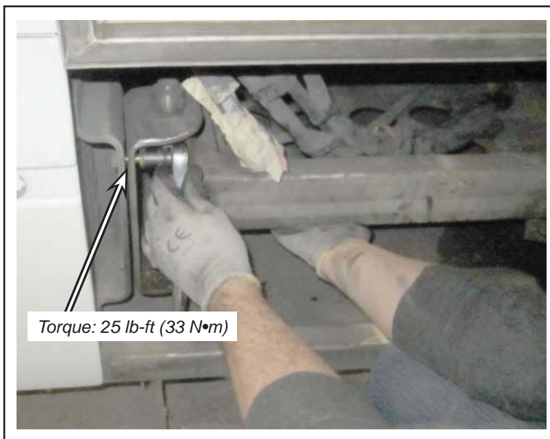
Figure 4 - Pivoting Tray Hinge
