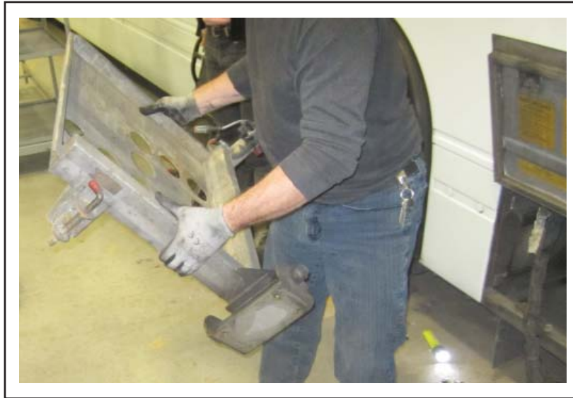
Figure 5 - Pivoting Tray Removed from the Battery Compartment
