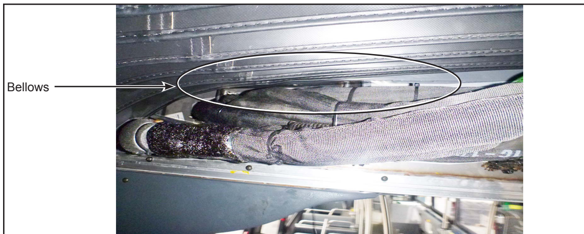
Figure 36 - Avoid Contact With Surrounding Components
