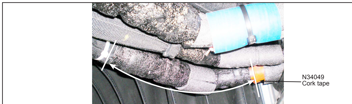
Figure 38 - N34049 Cork tape Installation
