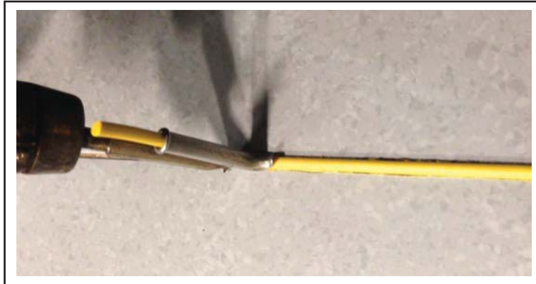
Figure 17 - A Good Weld Bead
