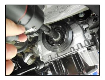
5. Remove and discard the crankshaft pulley. If necessary, use a harmonic balancer puller to remove the crankshaft pulley. In most cases, the puller will not be required.
