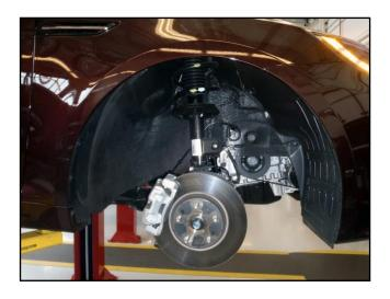
2. Remove the under-cover splash shield.
