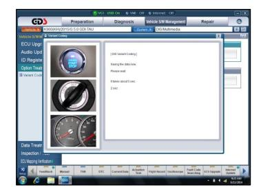
Once the GDS displays the "Save is completed" message, click on OK to complete the variant coding procedure.
